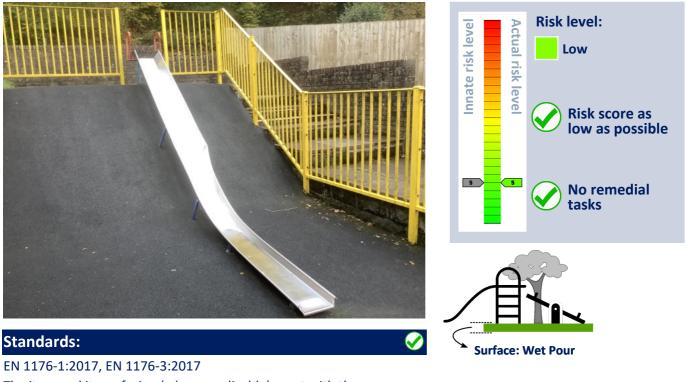
EN 1176-1:2017, EN 1176-3:2017 The item and its surfacing (where applicable) meet with the requirements of the relevant standards.
